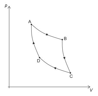
(a) Show, using the first law of thermodynamics, that during the process from A to B energy is supplied to the gas.
