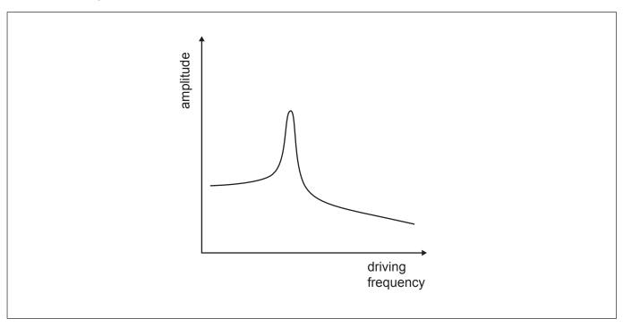
The graph shows the variation of the amplitude of oscillations with the driving frequency.
