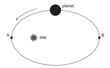
At point A the planet is closest to the star and at point B it is furthest from the star. As the planet orbits the star it has a moment of inertia  $I = mr^2$  where m is the mass of the planet.
